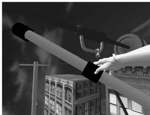
**FIGURE 13** Trainee is insulating the power line using an insulation cover.
