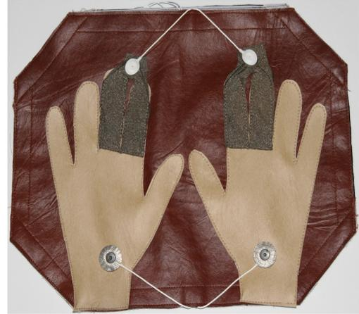
Figure 1: Experimental apparatus: at the top Electrolycras enable the acquisition of ECG using the index and middle fingers; at the bottom dry Ag/AgCl electrodes acquire ECG at the hand palms.
