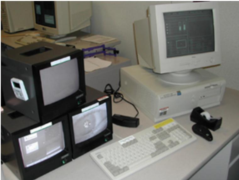
Figure 2. ISCAN eye tracker set up, with computer running tracking software (right) and three small monitors (left). The left small monitor shows the scene; the right small monitor shows the participants' eye with tracking information overlaid.
