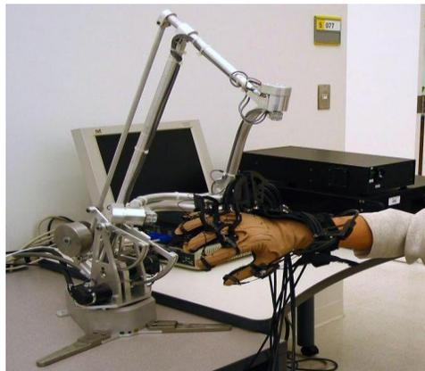
Figure 1: CyberGlove system used in our haptic-enabled rehab system
