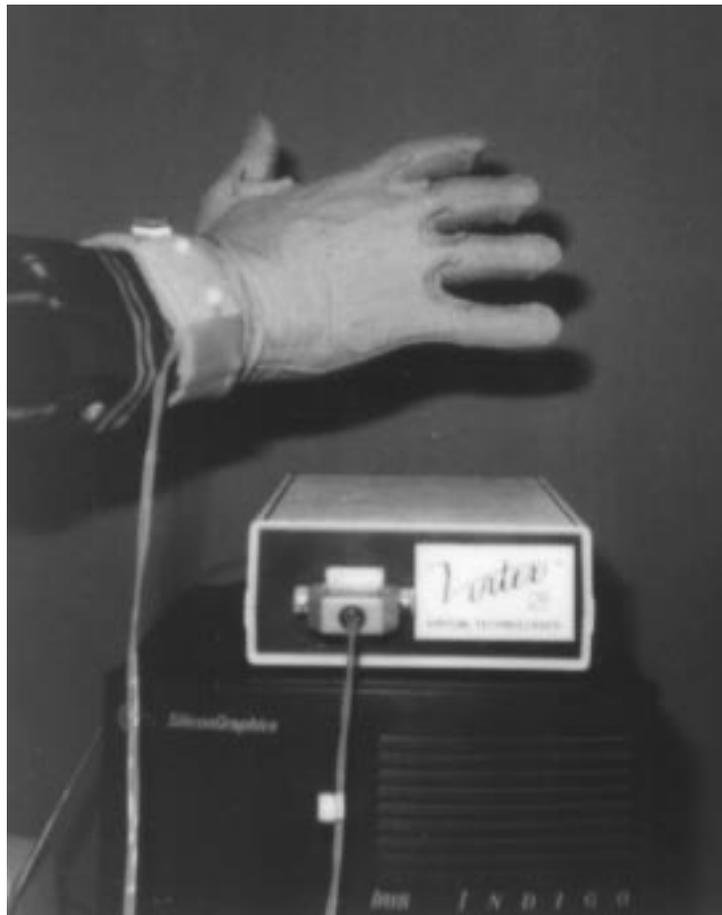
Figure 1: Virtual Technologies CyberGlove™
