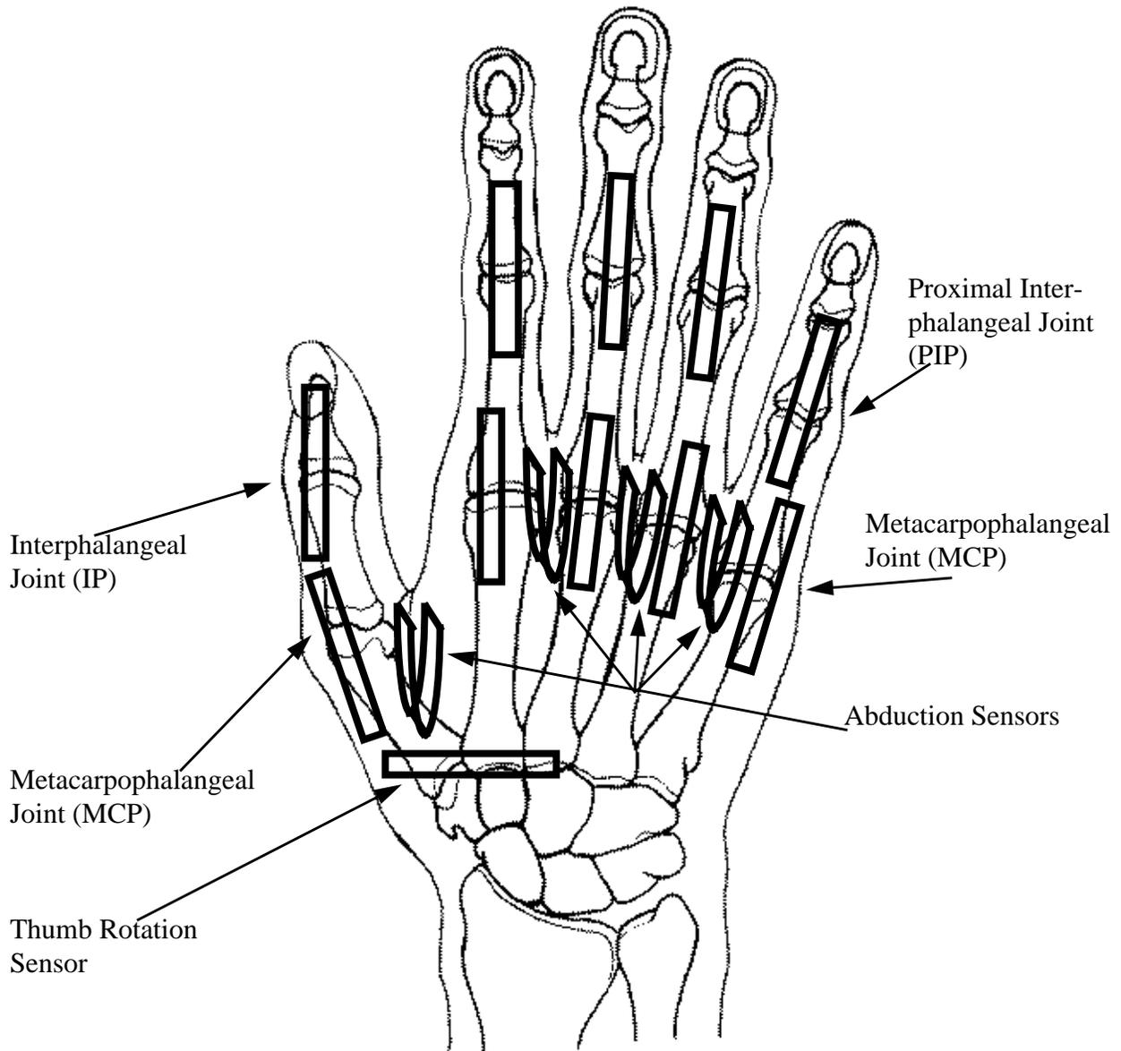
Figure 2: Sensors and Joints
