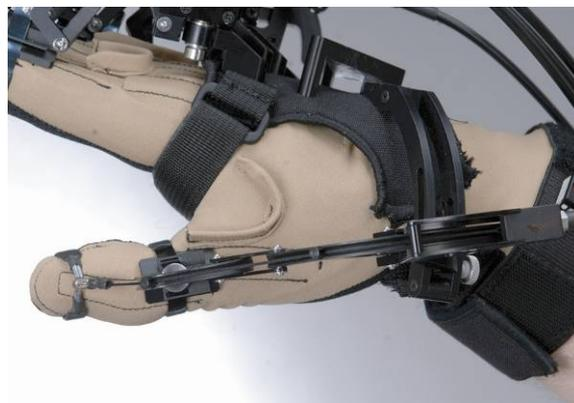
7. The next step is to ensure that the thumb assembly is properly aligned with the thumb as indicated in the Figure 13. This is achieved with the adjustment screw shown in Figure 14.
