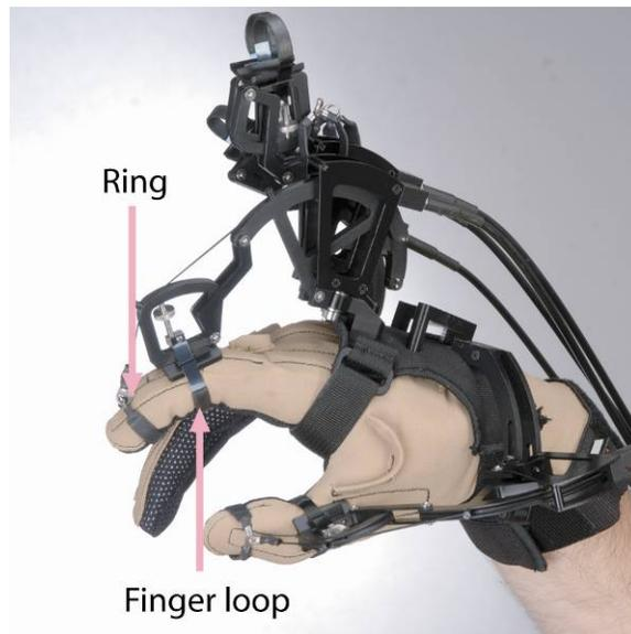
5. Slide all the finger loops onto the corresponding fingers. If they are too tight, loosen them using the thumbscrew. The force applicator rings should then be slid
