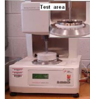
Figure 2. Paar Physica MCR 300 parallel disk rheometer.
