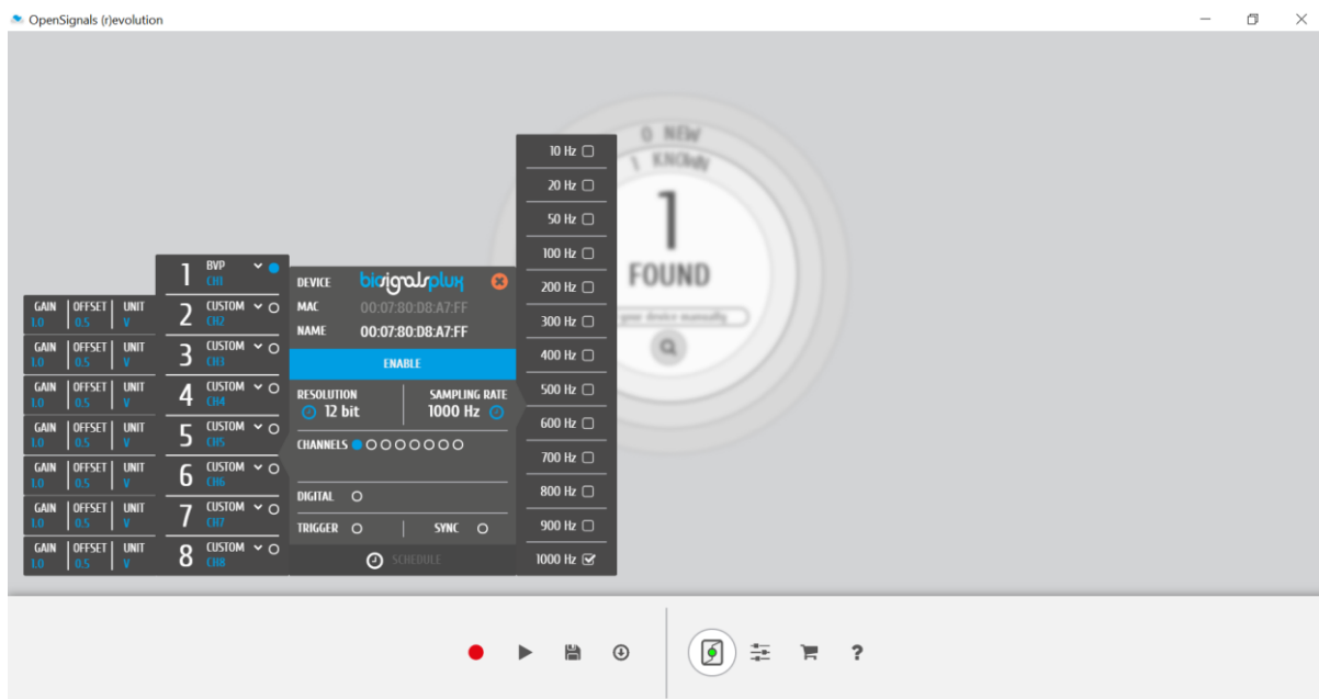
Figure 8: Set the channel type of the channel you have your BVP sensor connected to, to BVP .
