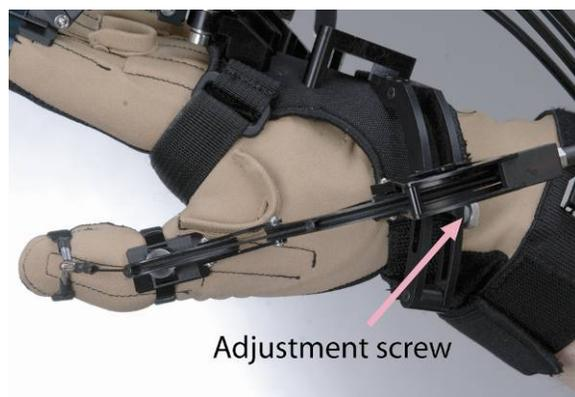
Loosening the adjustment screw will allow you to slide the thumb assembly in the slot so it can be aligned with the thumb.
