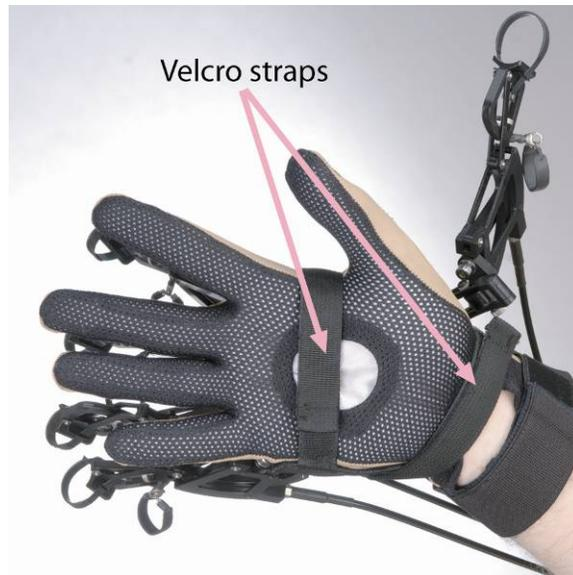
4. Tighten both Velcro straps as tightly as possible without making the fit uncomfortable. At this point, the backplate should be firmly and squarely positioned on the back of the hand.
