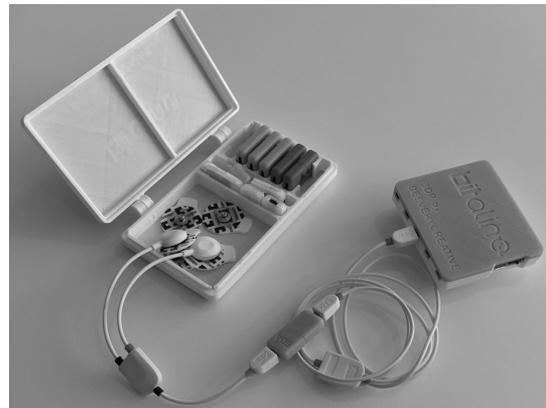
Fig. 2. BITalino or third party sensors can be connected by cable to the main board in any user-defined configuration (all the enclosures shown in the image are optional accessories).
