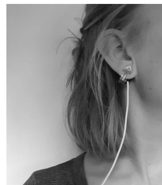
Fig. 4. PPG sensor positioning on the earlobe.
