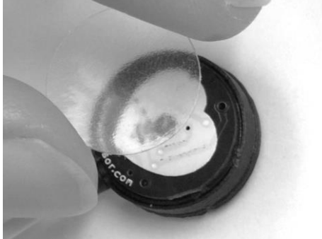
Fig. 5. PPG sensor vinyl sticker placement.
