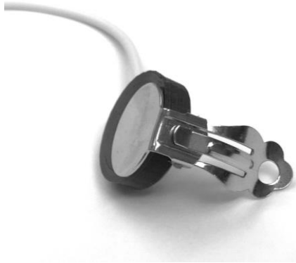
Fig. 11. PPG sensor placement of ear clip.
