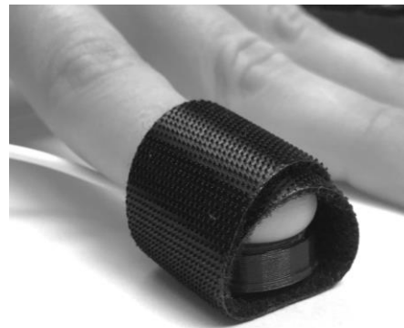
Fig. 8. PPG sensor fixation around the fingertip.
