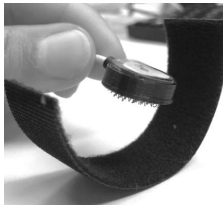
Fig. 10. PPG sensor fixation on fastening strap.
