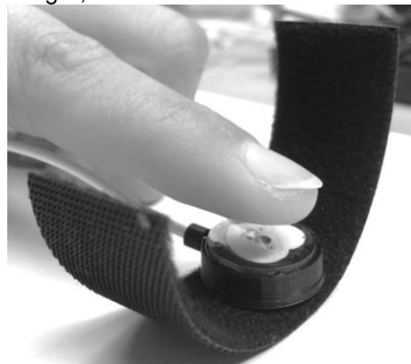
Fig. 7. PPG sensor placement on fastening strap.
