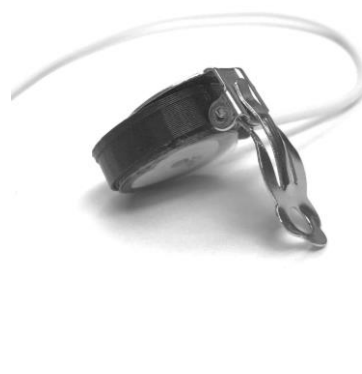
Fig. 12. PPG sensor fixation of earclip.
