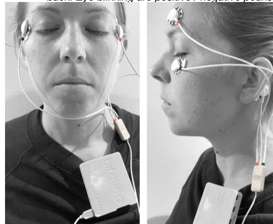
Fig. 4. Electrode Positioning – horizontal with IN+/- next to both eyes (left) and vertical with IN+/- above and below one eye (right) and both with REF behind the ear.
