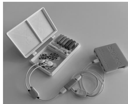
Fig. 3. BITalino or third-party sensors can be connected by cable to the main board in any user-defined configuration (all the enclosures shown in the image are optional accessories).
