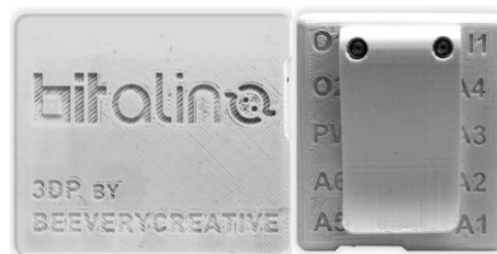
Fig. 2. Assembled BITalino Core with an enclosure for user-friendly applications. From up-left to down-left: O1, O2, PWM, A6, A5. From right-up to right-down: I1, A4, A3, A2, A1. See Figures 4 & 5 as complement.
