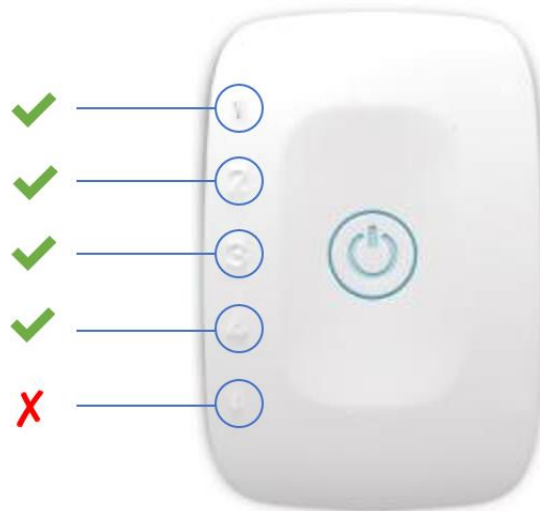
Figure 6: PZT compatible biosignalsplux channels (green checkmarks).
