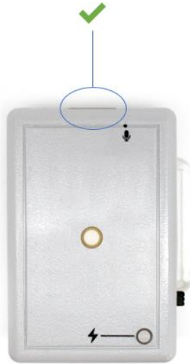
Figure 8: Connect the PZT to the analog input channel of the biosignalsplux Solo (openBAN).
