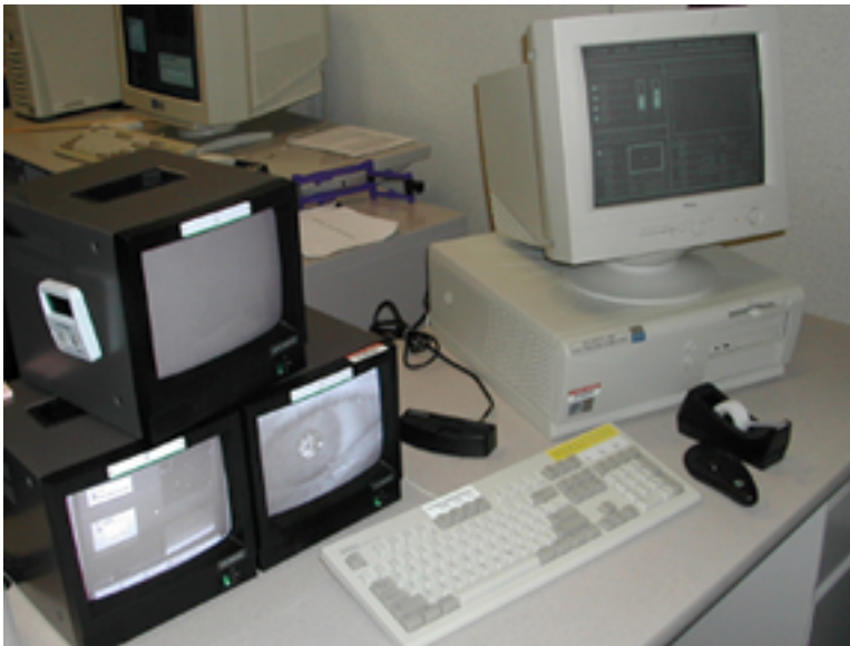
Figure 2. ISCAN eye tracker set up, with computer running tracking software (right) and three small monitors (left). The left small monitor shows the scene; the right small monitor shows the participants' eye with tracking information overlaid.
