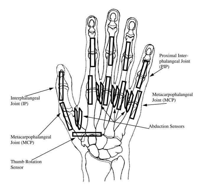
Figure 2: Sensors and Joints
