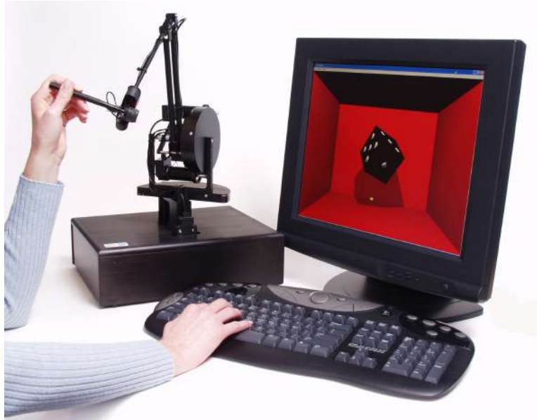
Figure 1.4. SensAble Technologies, Inc. PHANTOM haptic input/output device (reprinted with permission).
