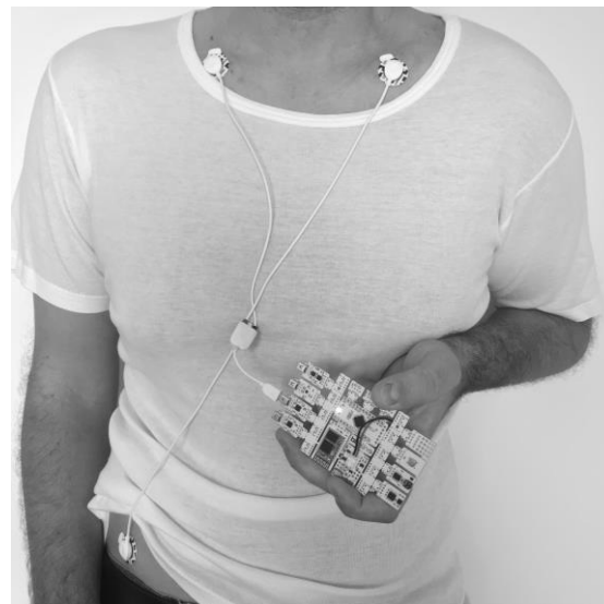
Fig. 3. Example of a 1-lead placement with IN+ & IN- on the collarbones and REF on the iliac crest.
