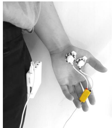
Fig. 4. Example electrode placement of the assembled version on the anterior side of the hand below the thumb.
