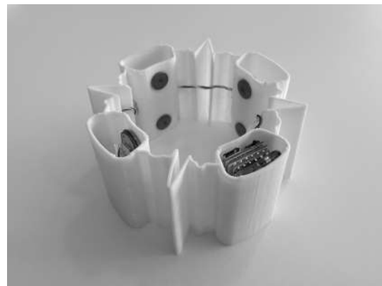
Fig. 2. BITalino Freestyle kits enable you to easily create wearables and miniaturized biosignal acquisition devices (some components in the image are optional accessories).
