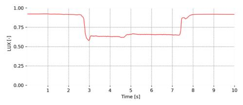
Figure 2: Typical unfiltered LUX sensor output while light change.
