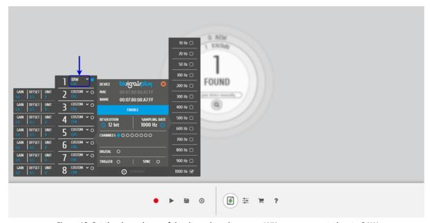
Figure 10: Set the channel type of the channel you have your LUX sensor connected to, to  $\it RAW$ .
