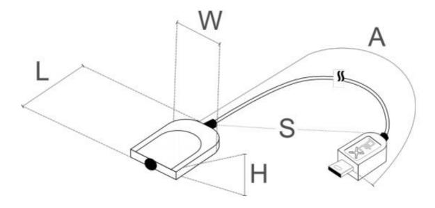
Figure 3: Physical characteristics of the standard Light (LUX) sensor.
