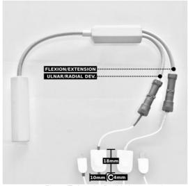
Fig. 1. Twin-axis, flexible beam goniometer.
