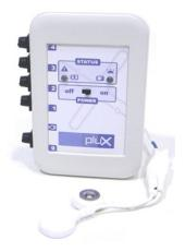
Figure 1. bioPLUX biosignal acquisition device
